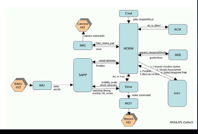
Surface navigation is the most complex module, comprising 21% of MER object code, 10% of MSL. How to manage its complexity?
